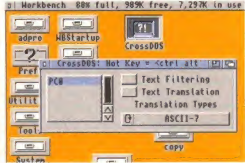
CrossDOS enables the Amiga to treat PC disks as if they were almost normal.
